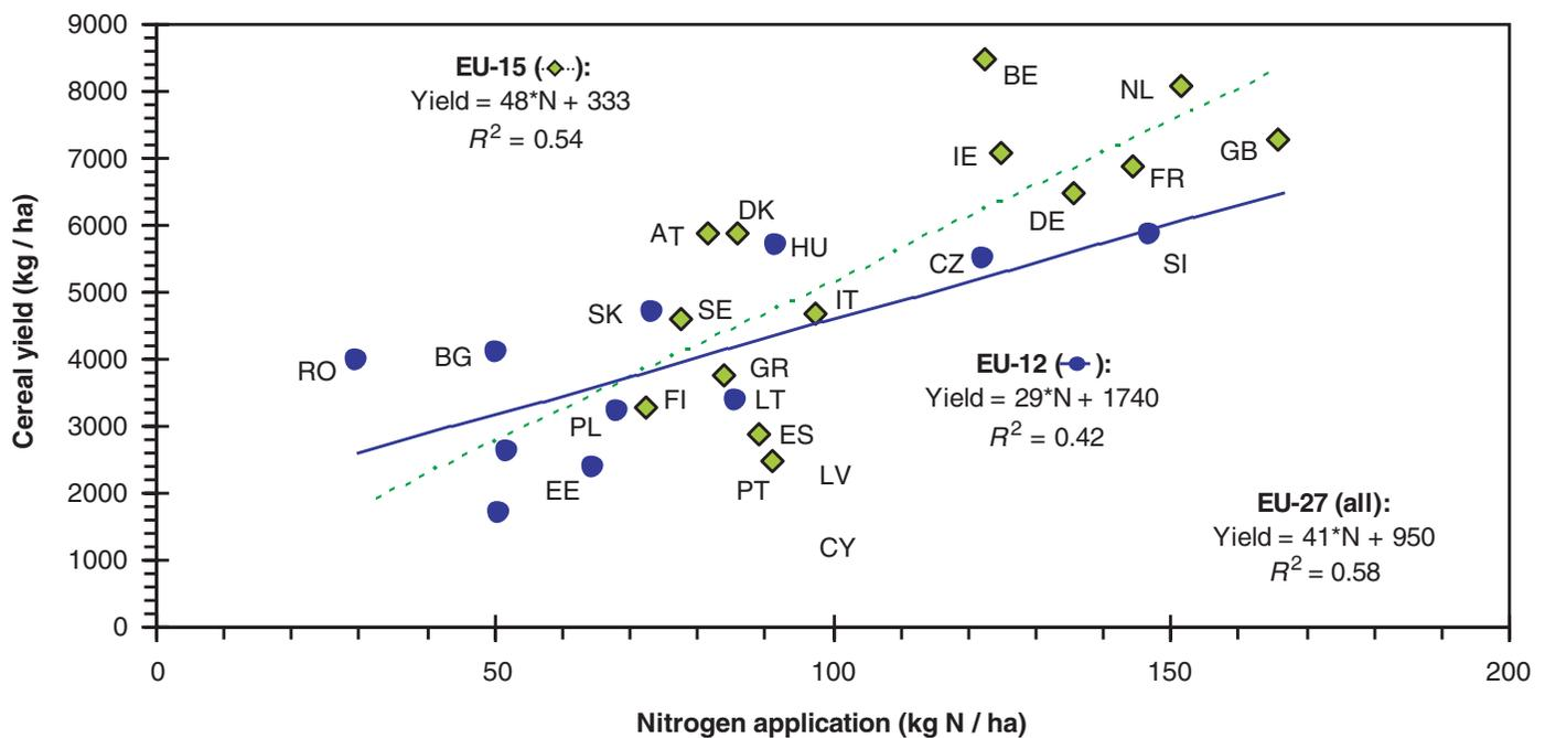
**Figure 3.7** Annual cereal crop yield vs. nitrogen application in the EU-27 countries. The slope of the regression lines, i.e. kg grain harvested per kg fertilizer N applied, is the apparent fertilizer N use efficiency, also termed the agronomic N efficiency. The slope does not differ significantly between EU-12 and EU-15 countries. Data from EFMA (2007).
