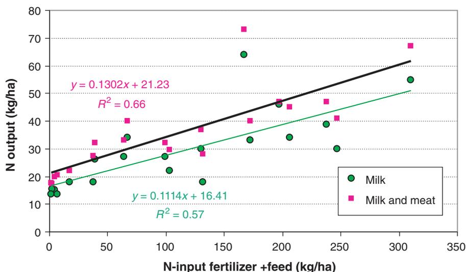
**Figure 3.16** N use efficiency on European dairy farms expressed as annual N output in milk and meat per annual N input in fertilizer + feed. Slope of the curves indicates gross NUE (based on data from Bleken *et al.*, 2005).
