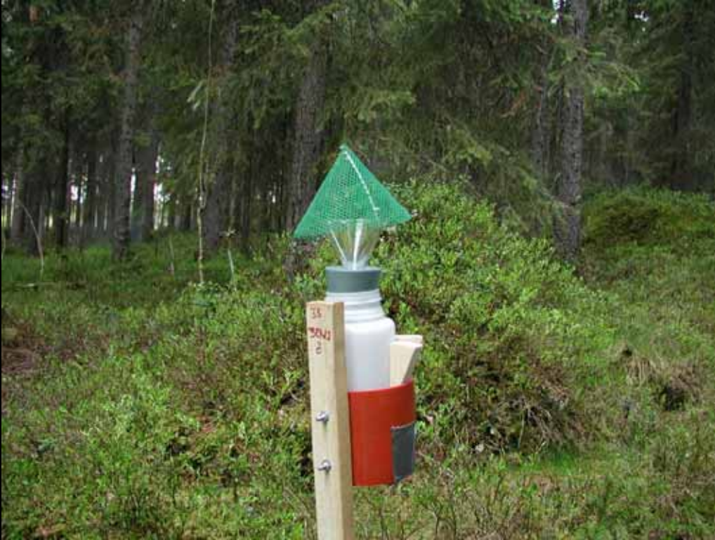
Rain in containers with acid holding solution
