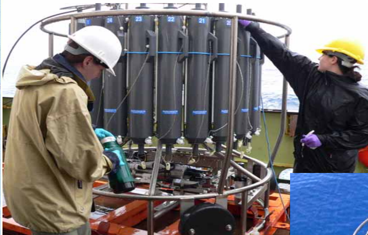
CTD-Rosette System 24 x 20 litre bottles Target the depths
